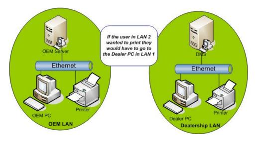
The above scenario is avoided if network 1 and network 2 are connected to a router to pass traffic between the networks. (see Figure 3.2, "Routed LANS")
