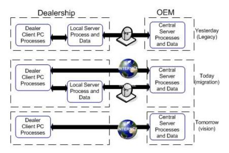
An external path to the data on the central server is required. Due to the volume of traffic required for dealership applications, the existing link to OEMs using the current satellite technology may not be adequate. Even small dealerships might find the delay of the medium unacceptable. That leads to the need to communicate over a faster and larger medium. The most likely choices include telephone services like a Digital Subscriber Line (DSL) and a T1.
