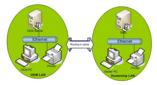
Routers with logical sub-interfaces contained on a single physical Ethernet interface can route traffic between sub-networks that exist in a switched environment. This allows traffic to pass or be filtered depending on the situation. Routers with multiple physical Ethernet interfaces can be used for non-switched and switched environments. Use routers with these capabilities to communicate between different sub-networks in a local environment.
