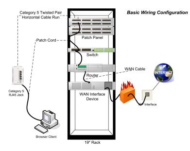
A sample wiring configuration is demonstrated above (see Figure 2.1, "Simplified Dealership Wiring"). This diagram represents the base configuration that allows a Personal Computer (PC) in the dealership to access the Internet. Dealer Management System (DMS) equipment, any satellite or OEM-specified equipment, and other dealership installed equipment comprising the remainder of the entire dealership network are not shown on this diagram.
